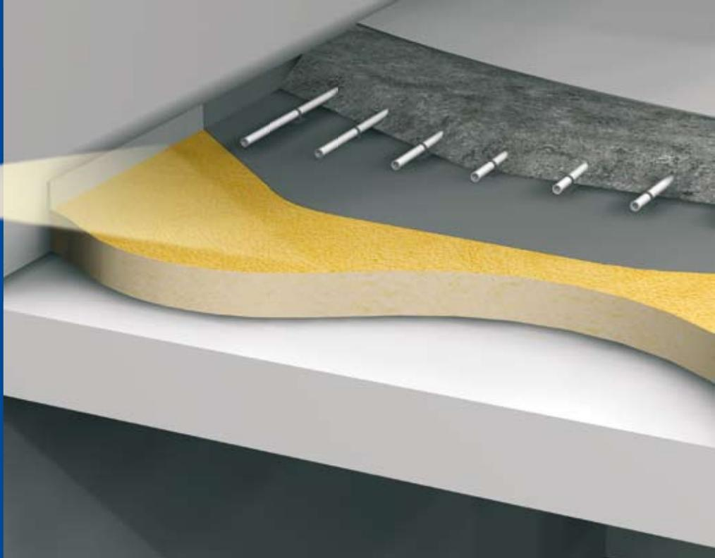
Thermal insulation above the floor slab is advisable where underfloor heating is installed. The insulating layer separates the heated and unheated areas inside a building and in this way reduces any loss of valuable heating energy. Even with rooms only used occasionally, insulation on top of floors with underfloor heating has benefits because the “cold” floor heats up more rapidly and no heat is passed into the floor slab.
