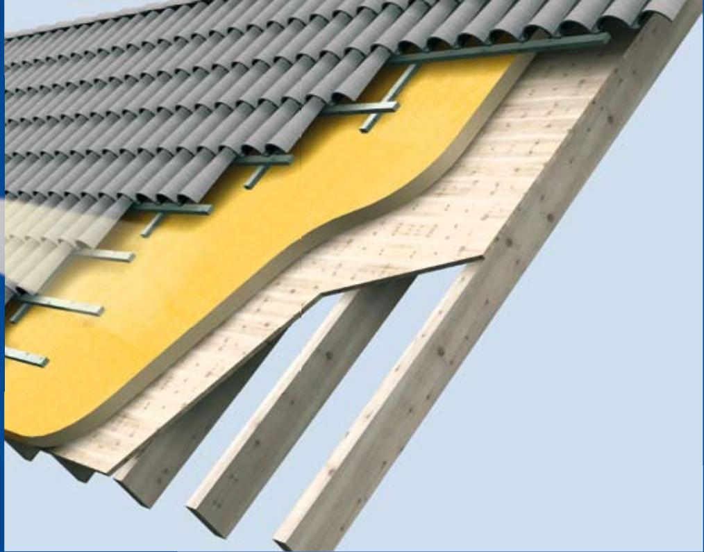
“Over-rafter” insulation means thermal insulation above the rafters. The insulating material is applied to the roof rafters from outside and only then is the roof covered – the rafters and roof board can still be visible from inside the room. Over-rafter insulation is an advantage if energy conservation and re-roofing are required. Ideal for attic rooms and loft conversions
