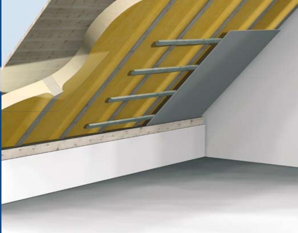
In times of rising energy costs and shortage of living area, loft conversions are becoming increasingly popular. Elastopor H can be applied from inside the loft space without the need for re-roofing, adding another room to the house, cost effectively.
